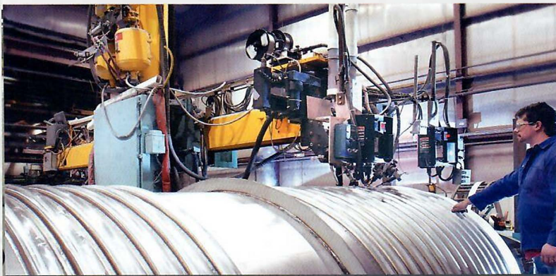
Full penetration half pipe – automated welding
