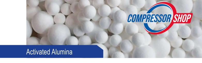
Activated alumina is a highly porous, ceramic compound that can absorb both gases and liquids without changing form or disintegrating.
